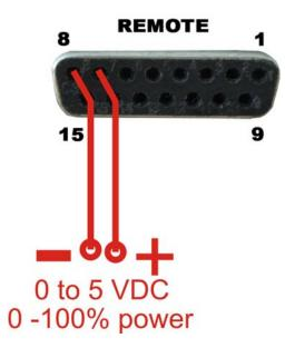
To enable control from PLC analog output, the client should open the generator and remove SMD resistor R14. In this case (after removing resistor R14) generator cannot be controlled with an external potentiometer, but it can be controlled with analog signal between pins 7 and 8 of the interface connector.
